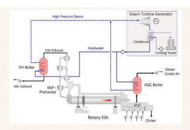
In the cement manufacturing industry, WHRS technology is capable of generating a significant share of electricity needs using waste heat. WHRS is a mature technology, with more than 850 WHRS installations world-
